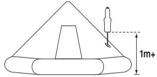
Alternatively, the SART may be attached directly to the liferaft canopy.
