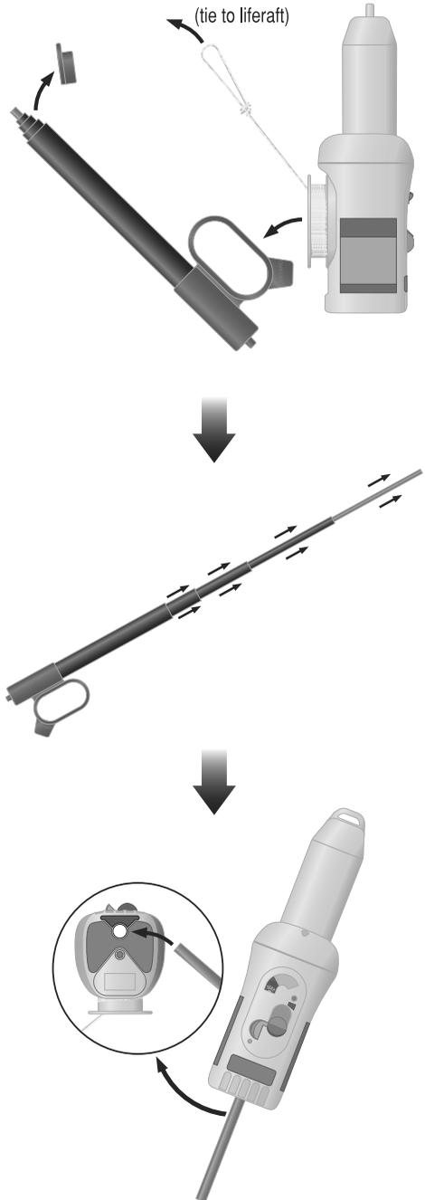
Raise the SART vertically and attach the pole to the liferaft. Most liferafts are fitted with suitable attachments to accommodate the SART pole.
